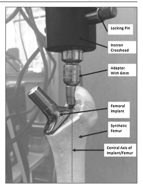
The implanted femurs underwent the same experimental setup as the synthetic bones. Testing was in a clockwise direction on the left, and anticlockwise on the right femur to ensure both hips were torqued in internal rotation. The data was analysed using SPSS (IBM SPSS Statistics, version 20) using a Mann–Whitney U test as data was not found to be parametric.
