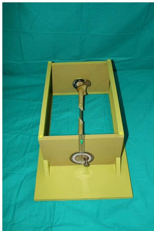
Fig. 1 Pediatric femoral fracture model mounted in wooden frame
