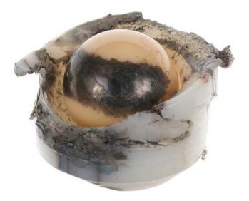
Fig. 6 Erosion of the polyethylene liner and resulting metalosis and staining
