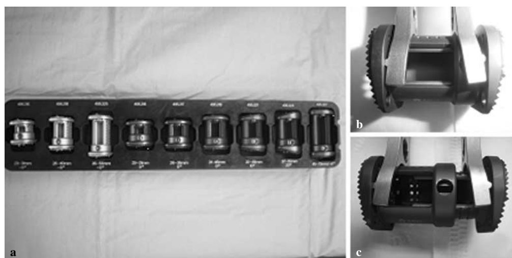
Fig. 1a-c Synex vertebral body replacement system (Synthes, Umkirch, Germany). a Operating kit with different sizes. b Close-up of the neutral state. c Extended state
