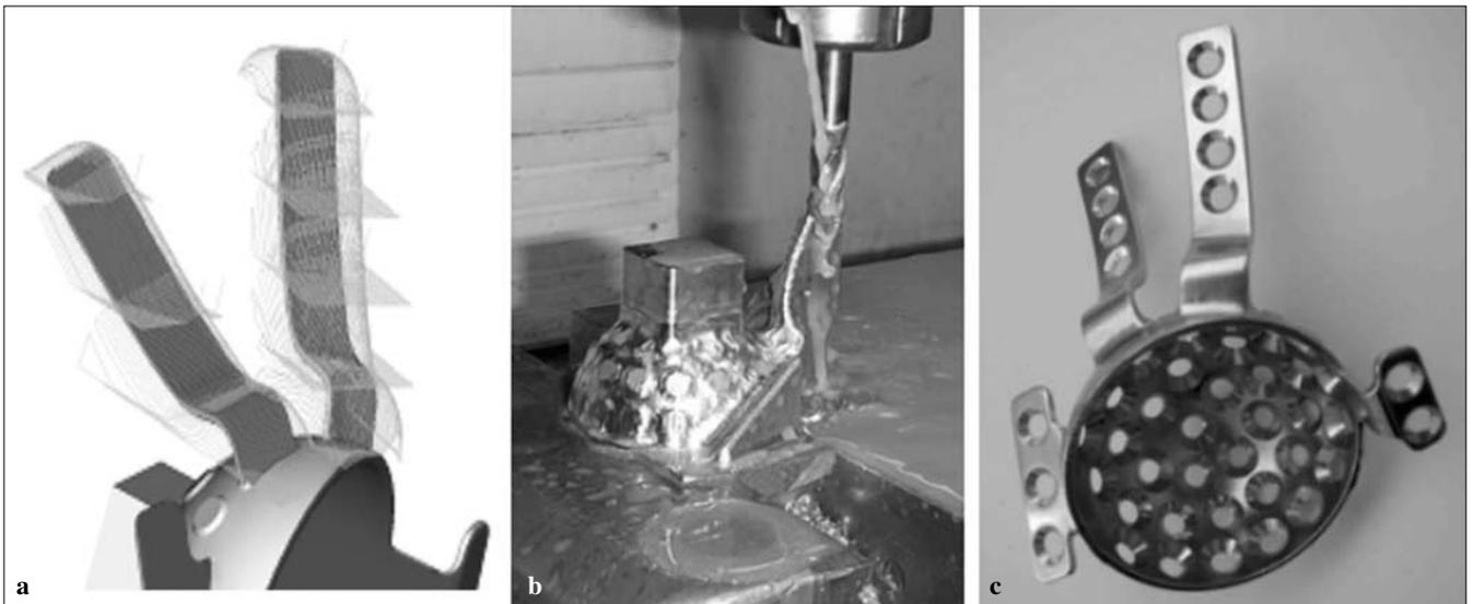
**Fig. 5a-c** The stages of cage manufacture in the CAM system. **a** Generated tool path. **b** Milling on CNC machine. **c** The manufactured cage
