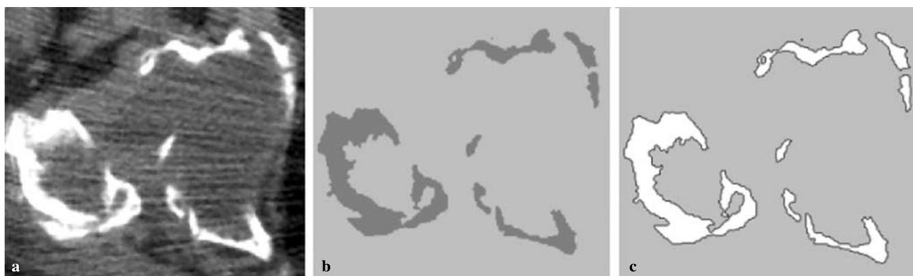
**Fig. 2a-c** Bone contour detection in one of the CT scans. **a** CT image. **b** Detected bone tissue of the determined radiological density. **c** Contours of the detected areas
